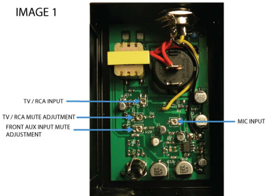
**NOTE:** the Adjustment Pots are delicate and will turn 360 degrees so it is important to have the unit connected and working when making fine adjustments
